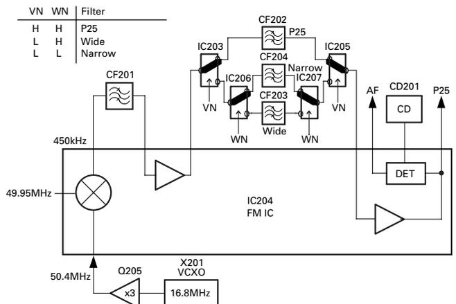
Fig. 3 Wide/Narrow/P25 switching circuit
