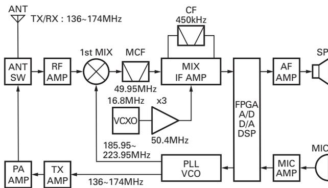
Fig. 1 Frequency configuration
