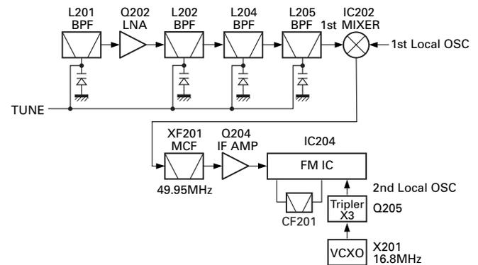
Fig. 2 Receiver section
