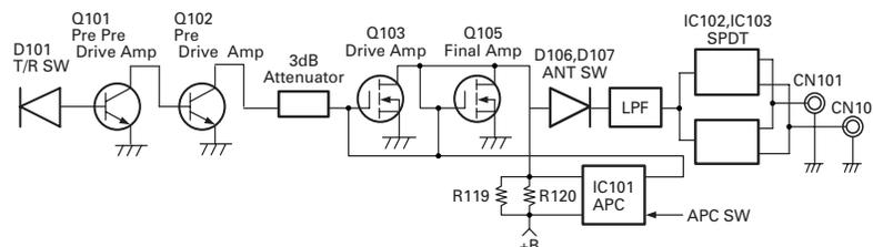
Fig. 7 Transmitter circuit
