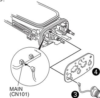
4. Pass the volume, channel switch, VOL/CH FPC and CONTROL-TOP FPC through hardware fixture holes, then bring the hardware fixture into contact with the chassis and fix it with a screw 5.
