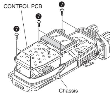
2. On the reverse side of the CONTROL PCB ⑧, remove the cord ASSY and each FPC from the connectors (CN601, CN604 (K2 and K3 models only), CN752, CN753) of the CONTROL PCB.
