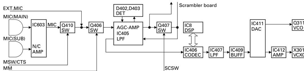
Fig. 6 Audio band and Base band circuit
