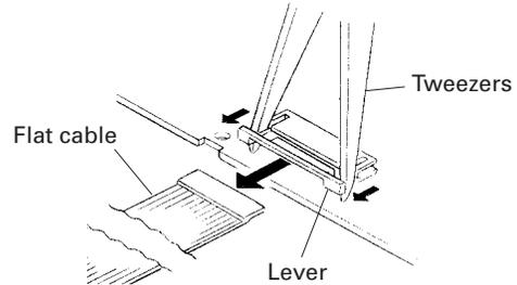
2. Gently rise up the connector lever in the direction of the arrow with a flat-head screwdriver or tweezers. (CN603)
