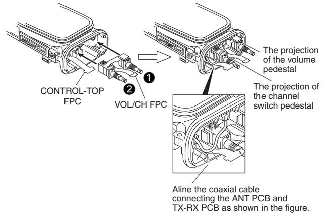
3. Pass the coaxial cable 3 of the antenna receptacle through the round hole of the hardware fixture 4, then insert it into the coaxial connector (MAIN (CN101)) of the TX-RX PCB.
