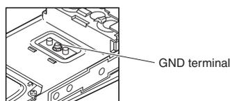
2. Tighten the two screws from the TX-RX PCB side.
