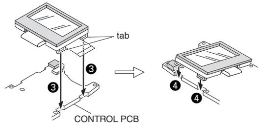
3. Insert the FPC into the CONTROL PCB connector (CN751) ⑤.
