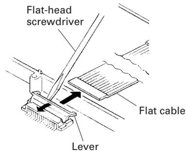
3. Gently depress the connector lever in the direction of the arrow with a flat-head screwdriver or tweezers. (CN902, CN903)
