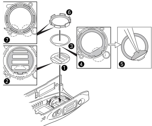
5. Verify that the packing does not ride on the rib of the case.
